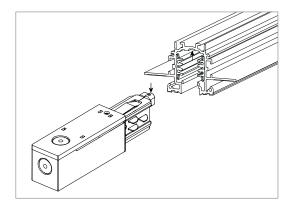
• The live end feed is equipped with a mechanical key to ensure the correct insertion into the track. This is to assist in the accurate wiring of the system.
